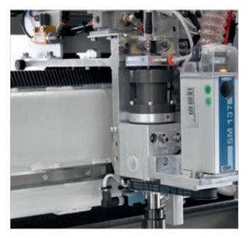
The operating head is equipped with a system that automatically manages the cutting pressure and ensures that the roller apply the proper force for the entire duration of the cut. The management of the axle speed and the high quality of all of the electronic and mechanical components enable machining times to be optimised, ensuring flexibility and dynamism.
