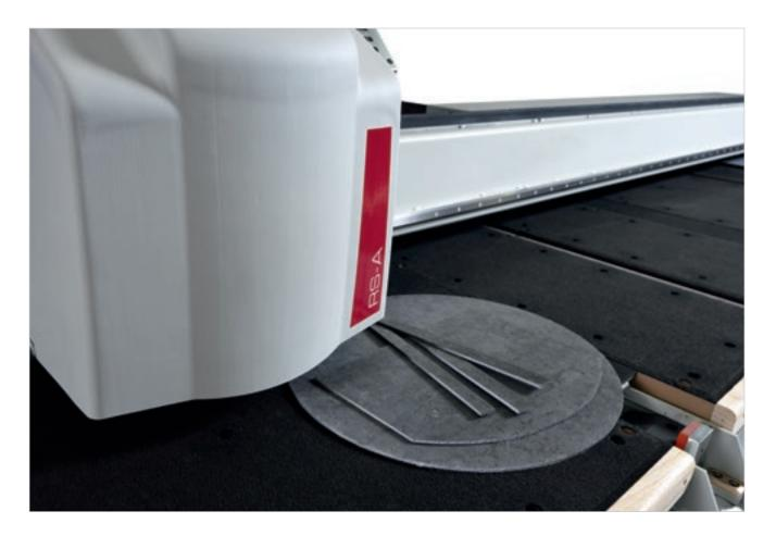
Biesse expands the limits for cutting low-thickness ceramic materials with new technology developed to perform the precision cuts typical of interior design (cladding for interiors and floors), counter tops, and construction (ventilated façades, stairs, thresholds, and windowsills). The Genius cutting table is easy to use and reduces waste. The main functions (cutting, breakout and loading/unloading, for example) are all included in the basic machine.
