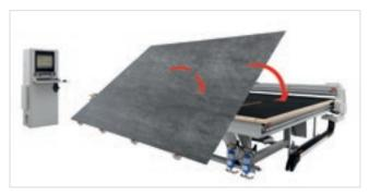
The retractable feet automatically move to the safety position before the cutting operation begins. The operating head automatically begins the cutting cycle.
