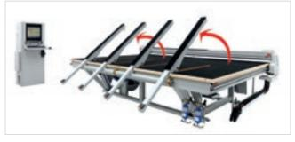
The machine operator manually positions the sheet of material on the tilting table.
