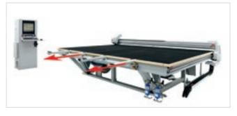
The arms of the tilting table automatically move back into the load position.
